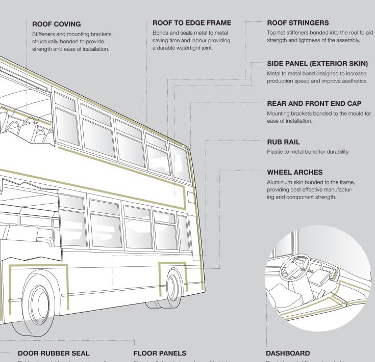
Rubber to metal bond provides weather resistance.
